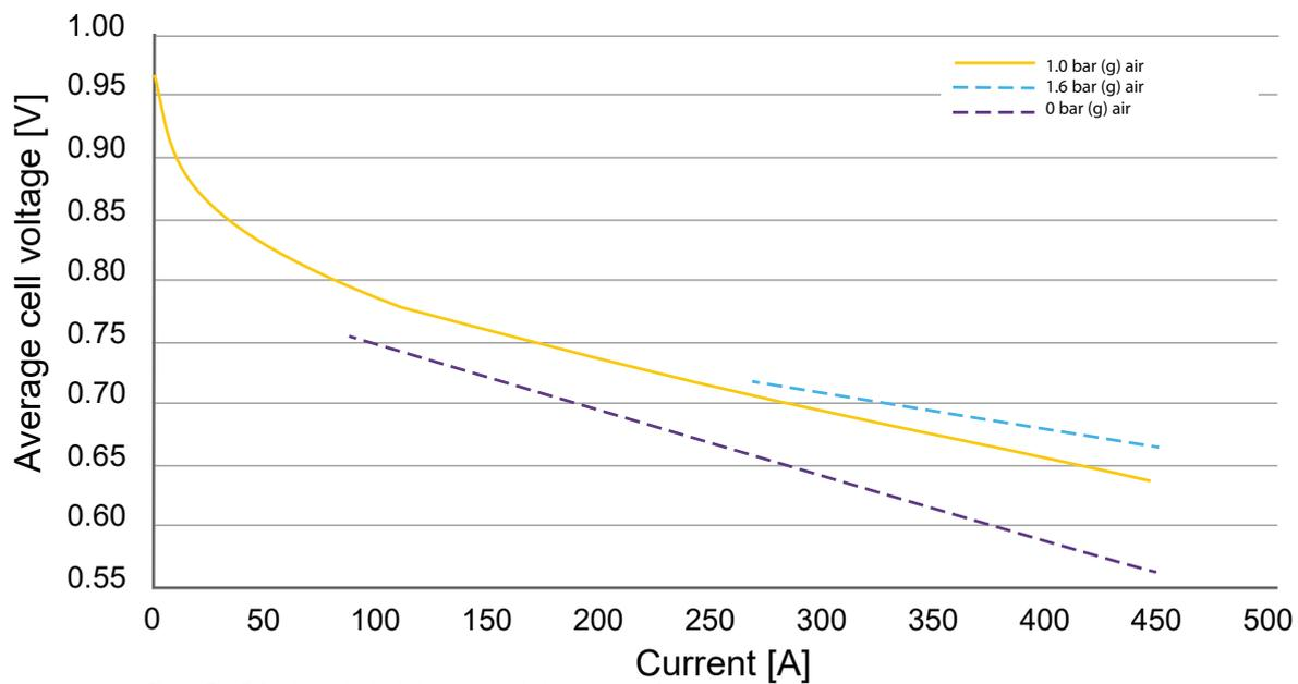
Figure: The P Stack standard polarization curve incl. pressure performance.<sup>iv</sup>
